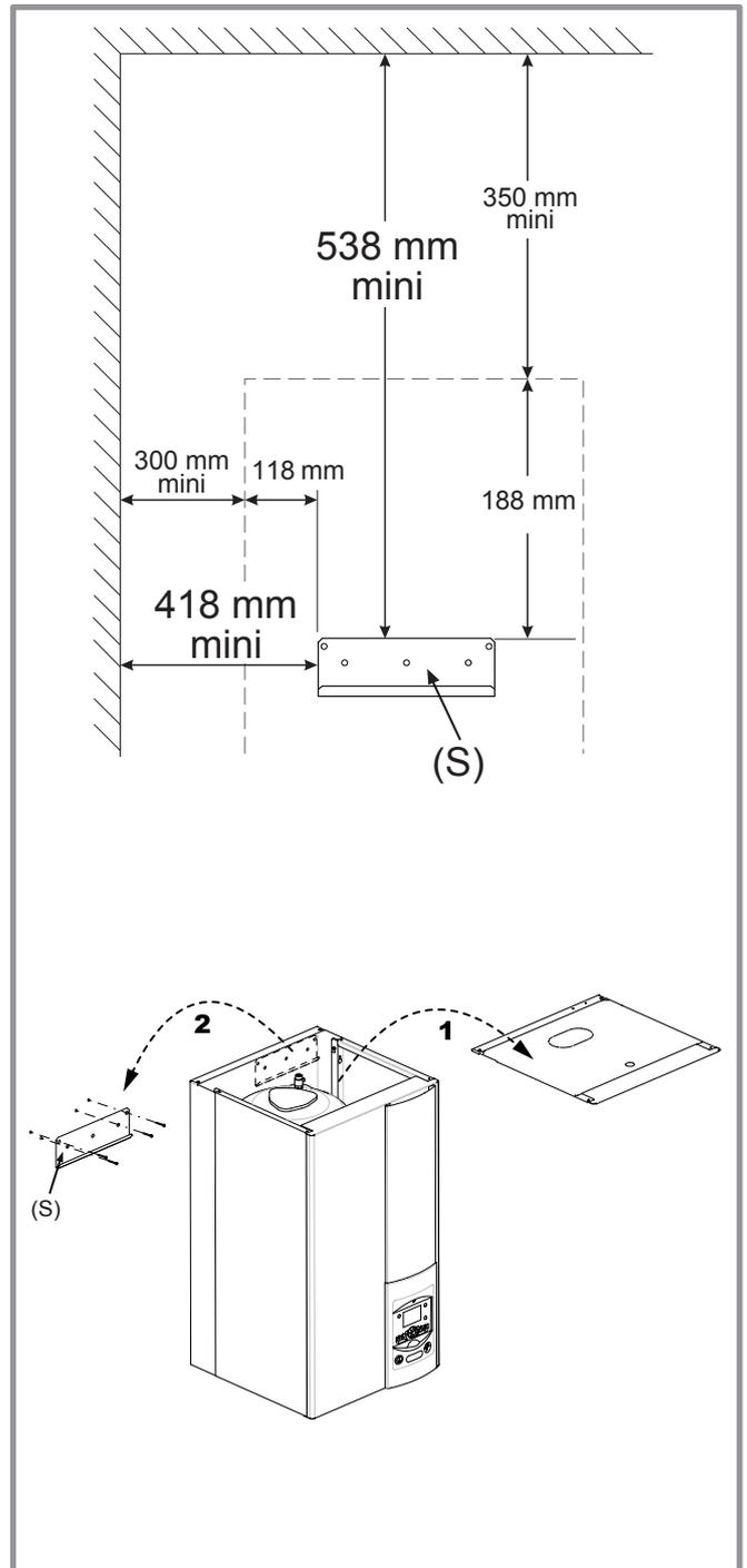
figure 17 - Fixation du support
