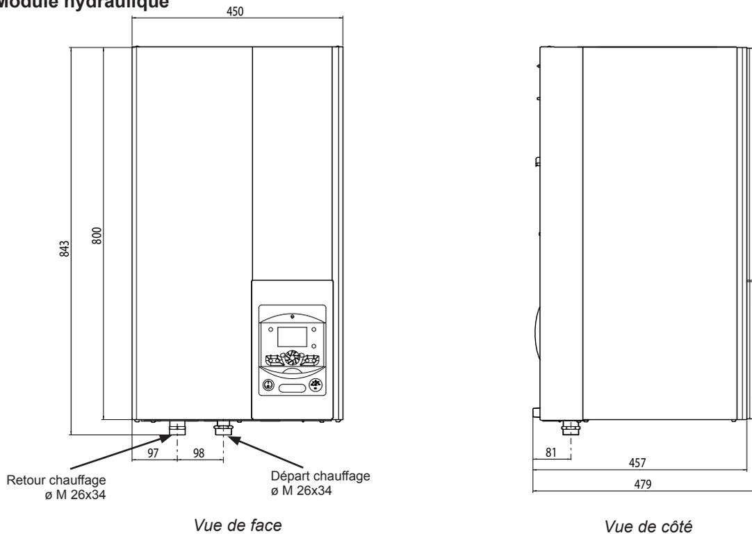
figure 4 - Dimensions en mm
