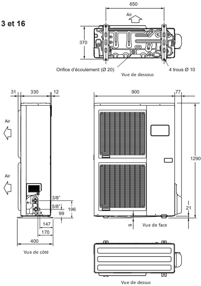
figure 3 - Dimensions en mm
